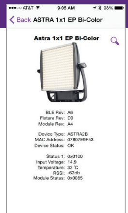
System information for a single fixture
